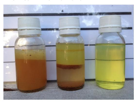
**Suspended Particulates** - can consist of mineral and metallic dusts from atmosphere, pipes & tanks, plus degrading fungal colonies.
